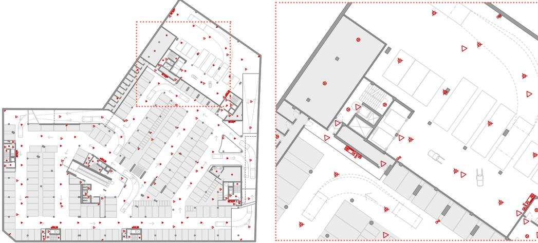
The bottom section displays two architectural floor plans of the same building. The left plan shows the entire layout with a dashed red box highlighting a specific area. The right plan is a zoomed-in view of this area, showing a staircase and several rooms. In this plan, fire extinguishers are marked with red icons and emergency lights with red triangles. The text to the right explains the placement criteria for these items.
