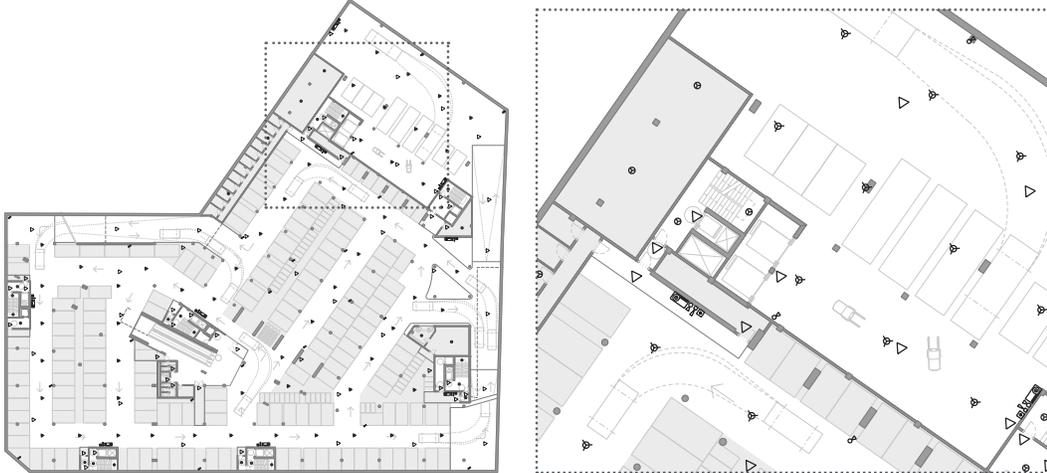
The top section displays two architectural floor plans of a building. The left plan shows the entire layout with a dashed black box highlighting a specific area. The right plan is a zoomed-in view of this area, showing a staircase and several rooms. In this plan, fire extinguishers are marked with black icons and emergency lights with black triangles. The text to the right explains the placement criteria for these items.
